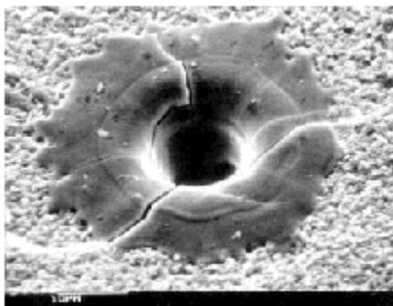
Figure 7. Charge cluster borehole into lead glass. Hole is about 10 micron diameter. Penetration is about 1mm per kV. The slowest speed clocked has been 1 cm in 50 nanoseconds. With an estimated 100 billion electrons carrying 100,000 positive ions, the kinetic energy exceeds 180 microjoules. It has been suggested that a Casimir effect pushes them together, overcoming Coulomb repulsion of like charges. (photo credit: Ken Shoulders)
